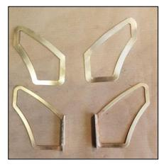
Here we have the frame parts ready, note that the newly cut frames are thicker in section, they are about 0.5 mm deeper where the window sits, the outside edge hasn't been filed to size yet, I'll do that once the glass is fitted.
