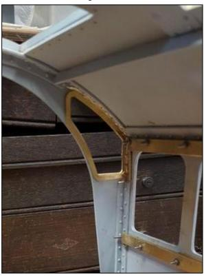
trying to remove the top bolt past the roof overhang would be a little problematic so I have used the two top holes as per Don's drawing but will use the one bolt for the bottom mounting bracket as per prototype, I have changed both brackets a little to accommodate this. The two unused bottom holes will be filled later before painting.
