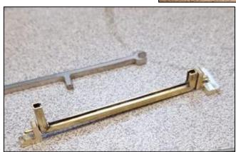
drilled the ends of the frames to solder in a short length of brass rod (cut to length later) I then machined the right-angle into the brackets required, before fitting, the corners were filed round and the mounting holes were drilled.
