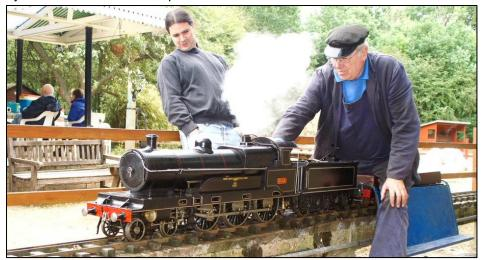
chairman, Sir Gilbert Claughton. Nigel Thomson of the Erewash Valley Model Engineers has brought his model of that engine to us on a number of occasions. The inside valves are actuated by rocking levers ahead of the cylinder bock, like many GWR engines, but with the valve gear on the outside.
