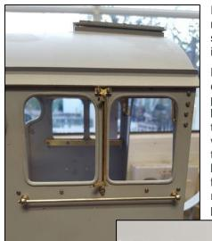
I also machined a semi-circle into the middle of the top bracket so that it was a snug fit up against the single bolt which is where the prototype holds the bracket.
