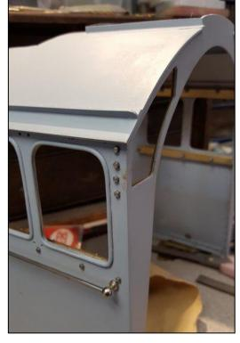
right-angle to the window frame and flush with the inside of the cab sheet, lining up nicely with the vertical line of 4 bolts. I hope that all makes sense....one other thing is that it looks like there may be a hinge here too, I assume to open the window perhaps to wipe clean while in service. Since there is no way that a finger
